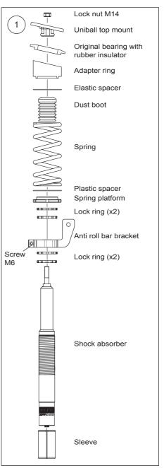
Fit and tighten the M14 lock nut by 60 Nm (44 ftlb) and hold the strut steady with a 6 mm allen key. Make sure you rotate the nut and not the top pin!
